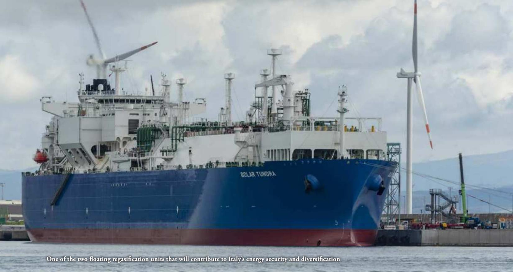
One of the two floating regasification units that will contribute to Italy's energy security and diversification
